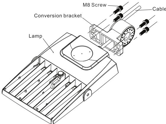
2. The cable passes through the conversion bracket and is fixed conversion bracket to the lamp with M8 screws.
