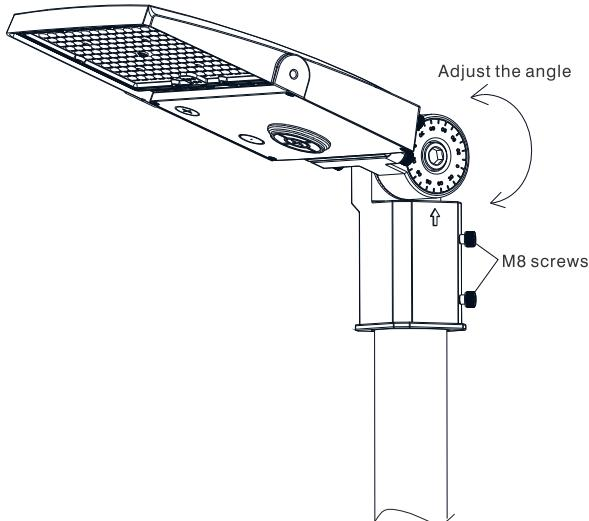
5. The wires are hidden inside the lamp pole; The lamp is fixed to the lamp ploe with M8screws. Adjust the light output angle of the lamp.
