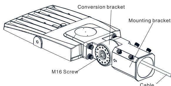
3. The cable passes through the mounting bracket; The mouting bracket and conversion bracket are fixed together with M16 screws.
