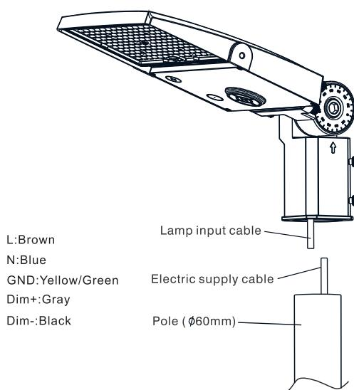
4. Connect the input line of the lighting fixture to the municipal power line.
